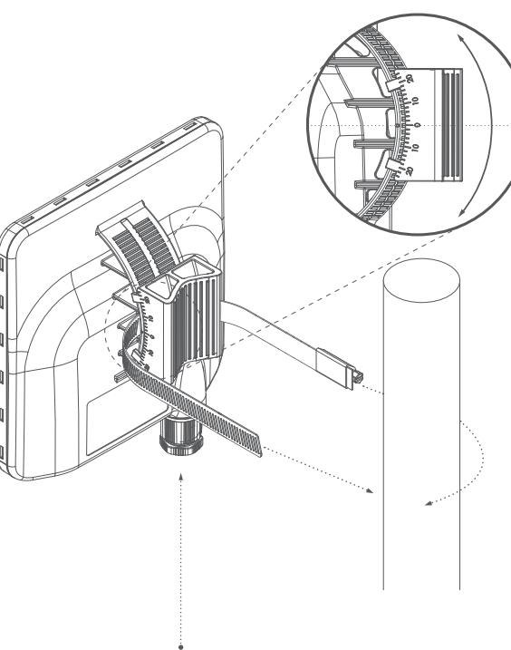
Device cable gland must be positioned vertically downwards
